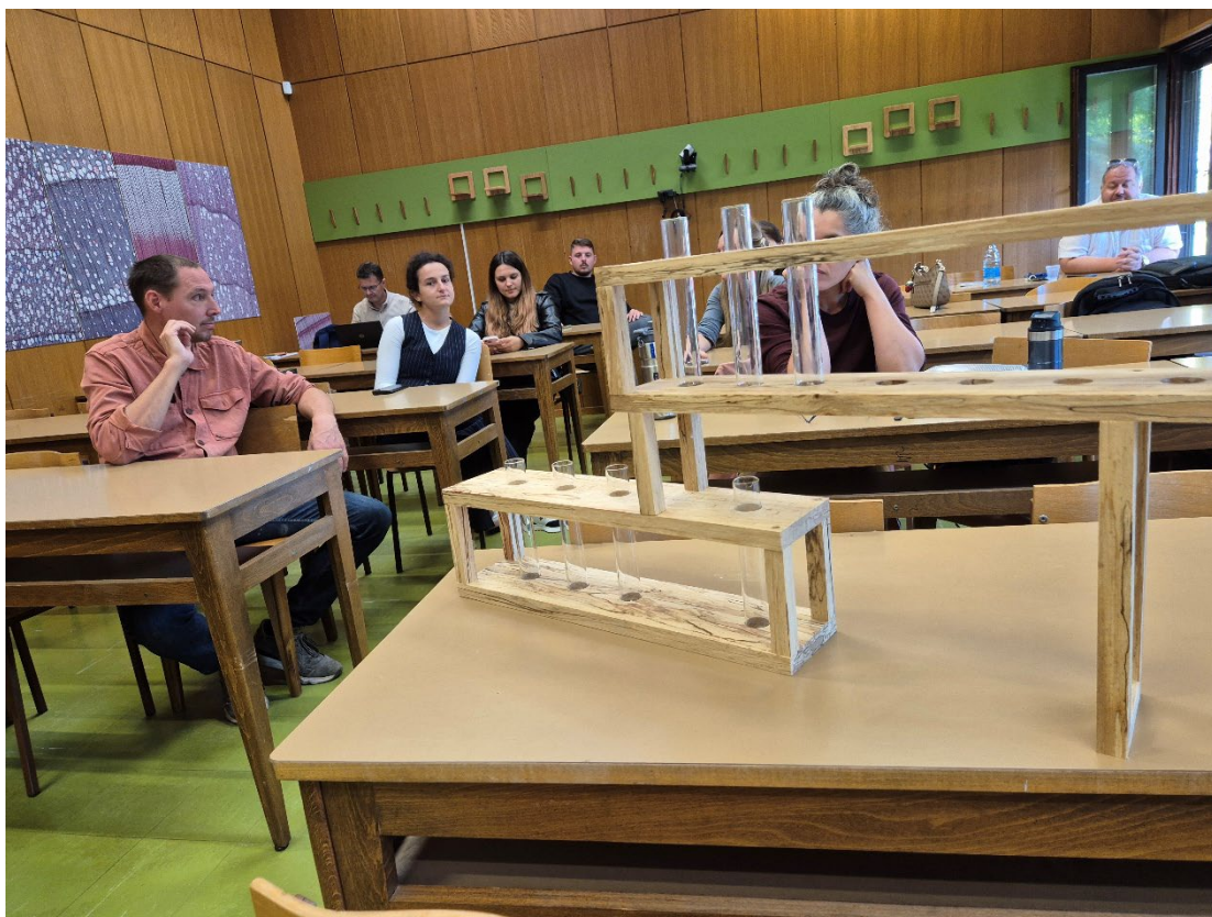
Figure 16: Prototype stands for seedling cultivation in test tubes, crafted from decayed coloured beech wood.
